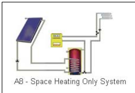
Figure 5.3: Space heating system (from: www.Valentin.de )
